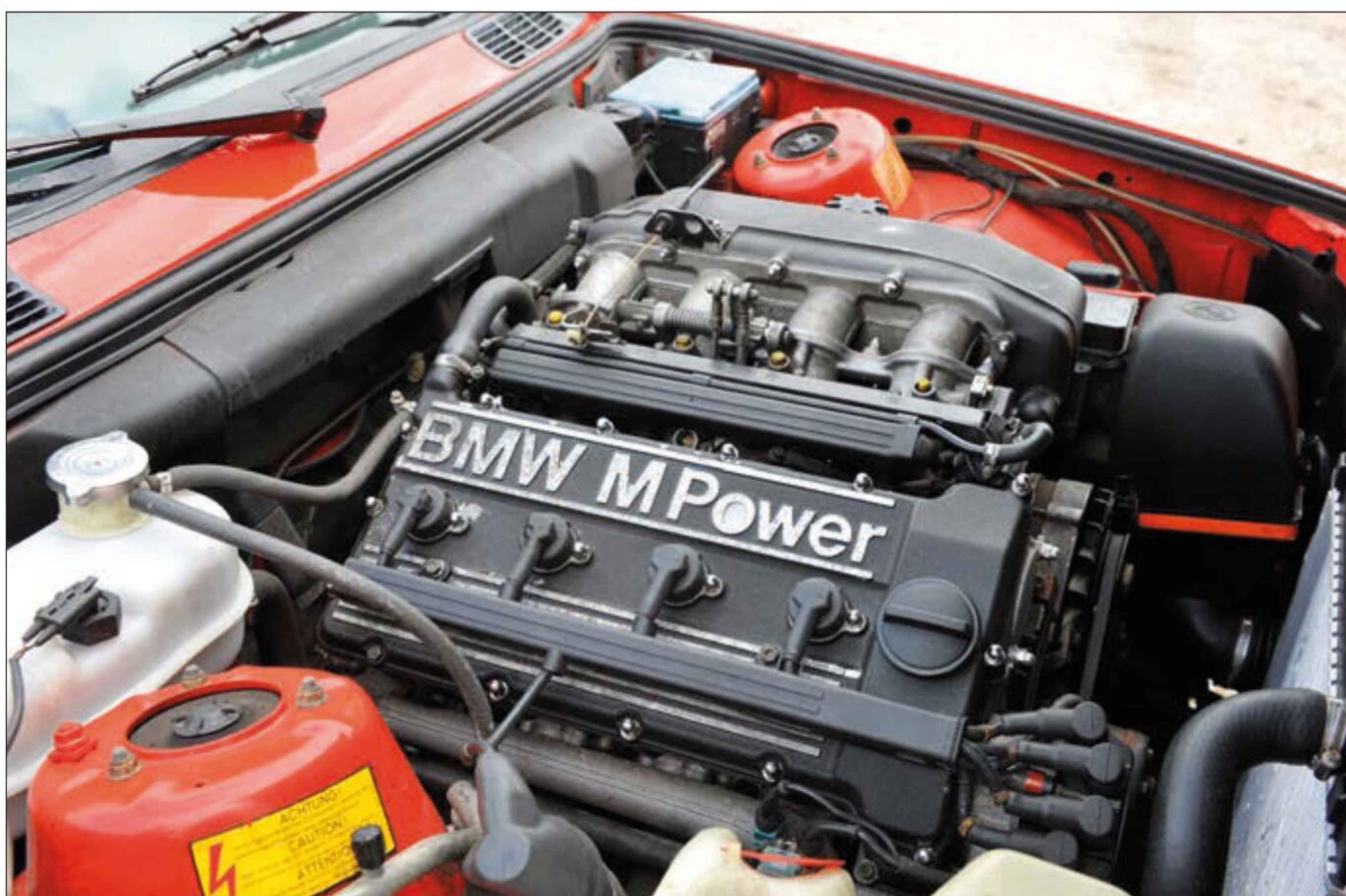
The four-cylinder, S14 engine powered the E30 M3 throughout its production life, albeit with a number of notable modifications along the way.
