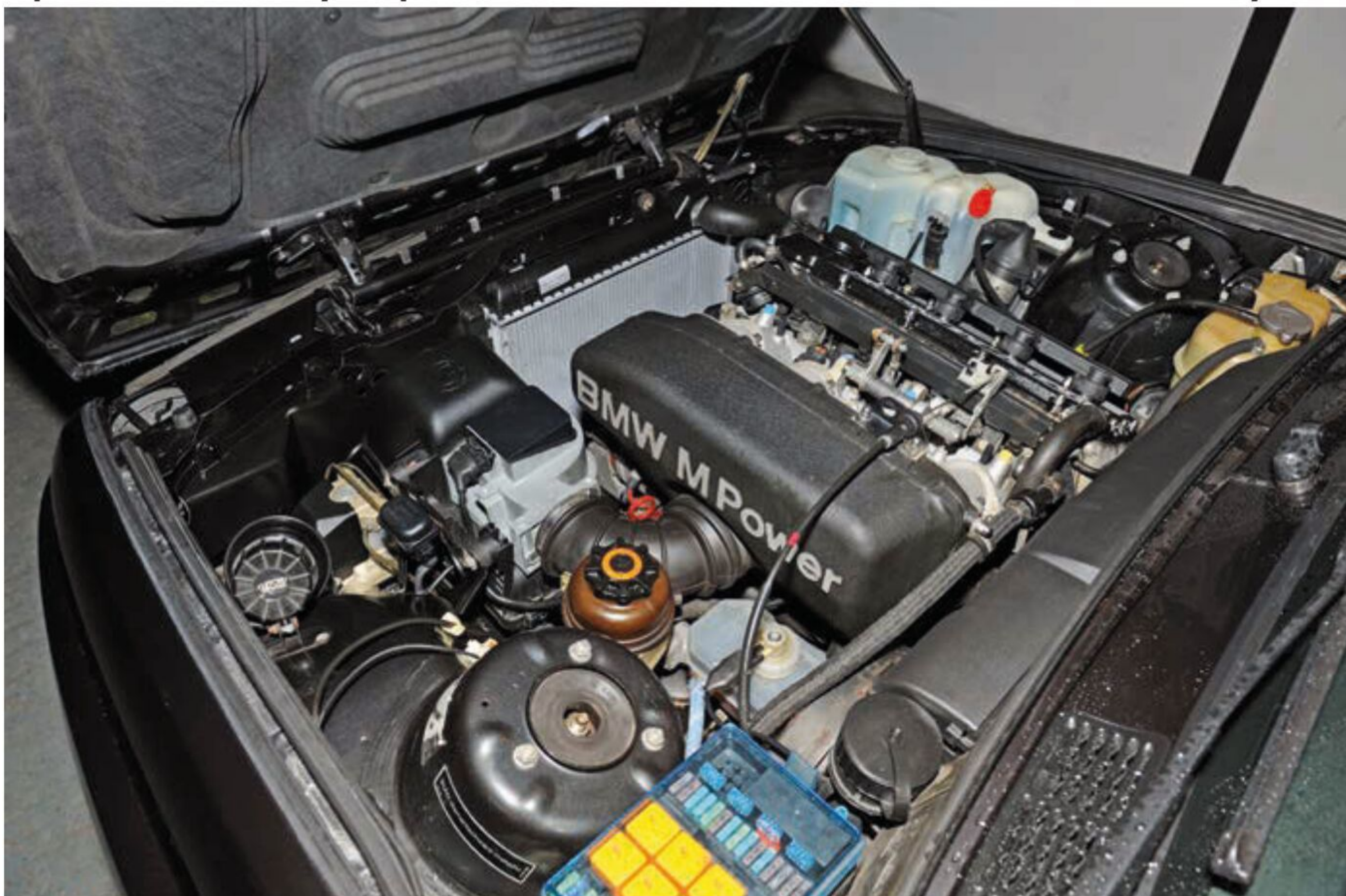
The M3's S14 engine was developed in house by BMW's M division. It uses head technology derived from the larger M-cars.
